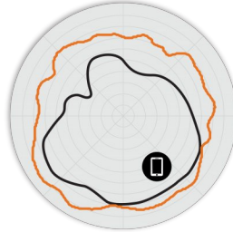
Figure 6. T670 5GHz Elevation Antenna Patterns
