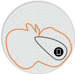
Figure 5. T670 2.4GHz Elevation Antenna Patterns
