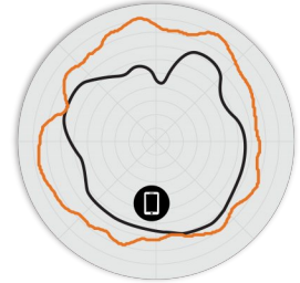
Figure 7. T670 6GHz Elevation Antenna Patterns
