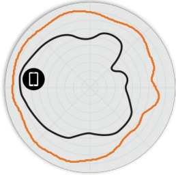
Figure 5. T670 2.4GHz Elevation Antenna Patterns
